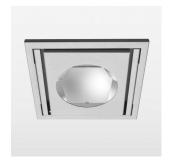
Recessed luminaire with LED, rated life of the LED L80/B10 > 50000 h, colour rendering index CRI > 70, chromaticity tolerance 2 SDCM (initial), reflector with oval light distribution pattern, swivel angle 30° luminaire housing sheet steel, powder-coated, silver, separate driver unit
