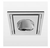
Recessed luminaire with LED, rated life of the LED L80/B10 > 50000 h, colour rendering index CRI > 70, chromaticity tolerance 2 SDCM (initial), reflector with circular light distribution pattern, reflector pure aluminium 99,99% in MIRO-Silver®,, swivel angle 30° luminaire housing sheet steel, powder-coated, silver, separate driver unit
