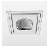
Recessed luminaire with LED, rated life of the LED L80/B10 > 50000 h, colour rendering index CRI > 70, chromaticity tolerance 2 SDCM (initial), reflector with circular light distribution pattern, reflector pure aluminium 99,99% in MIRO-Silver®,, swivel angle 30° luminaire housing sheet steel, powder-coated, white, separate driver unit
