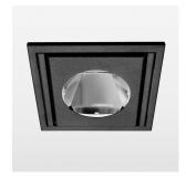
Recessed luminaire with LED, rated life of the LED L80/B10 > 50000 h, colour rendering index CRI > 70, chromaticity tolerance 2 SDCM (initial), reflector with circular light distribution pattern, reflector pure aluminium 99,99% in MIRO-Silver®,, swivel angle 30° luminaire housing sheet steel, powder-coated, black, separate driver unit
