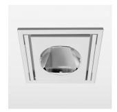
Recessed luminaire with LED, rated life of the LED L80/B10 > 50000 h, colour rendering index CRI > 90, chromaticity tolerance 2 SDCM (initial), reflector with circular light distribution pattern, reflector pure aluminium 99,99% in MIRO-Silver®,, swivel angle 30° luminaire housing sheet steel, powder-coated, white, separate driver unit
