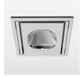
Recessed luminaire with LED, rated life of the LED L80/B10 > 50000 h, colour rendering index CRI > 70, chromaticity tolerance 2 SDCM (initial), reflector with circular light distribution pattern, swivel angle 30° luminaire housing sheet steel, powder-coated, silver, separate driver unit
