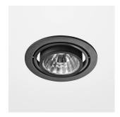
Recessed luminaire with LED, rated life of the LED L80/B10 > 50000h, colour rendering index CRI > 90, chromaticity tolerance 2 SDCM (initial), reflector with circular light distribution pattern, 99,99% pure aluminium, segmented and faceted, cardanic, incl. glass cover, sheet metal powder coated, separate driver unit
