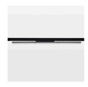
Surface-mounted luminaire with LED, rated life of the LED L90/B50 50000 h (tambient 25°C), colour rendering index CRI > 80, chromaticity tolerance 3 SDCM (initial), double asymmetrical light distribution pattern with slight horizontal brightening, Combination of asymmetrical PMMA lenses and 60 ° TIR lenses made of PMMA, luminaire housing sheet steel, powder-coated, black, locking mechanism to aligned in 15° steps, rotation angle 300°, In-Track-Adapter, On/Off, 220-240 V~ / 50-60 Hz
